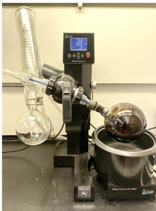
Fig 3: Weathering of AWWB using Rotatory evaporator.
