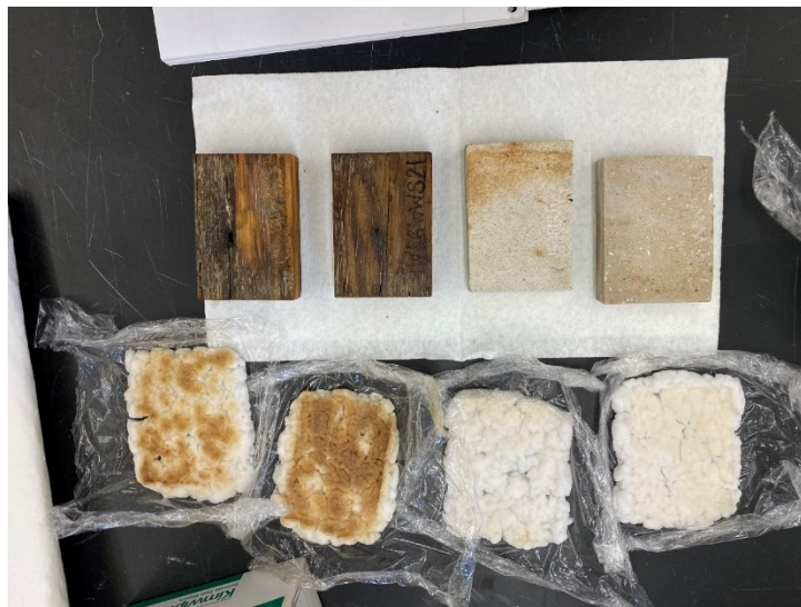
Fig. 5 - Poultice treatment on weathered yellow pine and concrete samples contaminated with WTI
