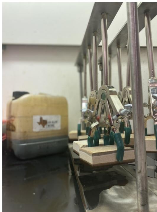
Fig 4: The concrete samples oiled with West Texas Intermediate are hung with clamps.
